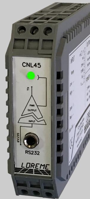
The CNL 45 is an isolated numeric transmitter powered by the 4-20 mA current loop, combining the ease of use of loop powered device with the flexibility of programmable converters.
